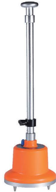
**APPLICATION:** Power cable main insulation fault pinpointing
