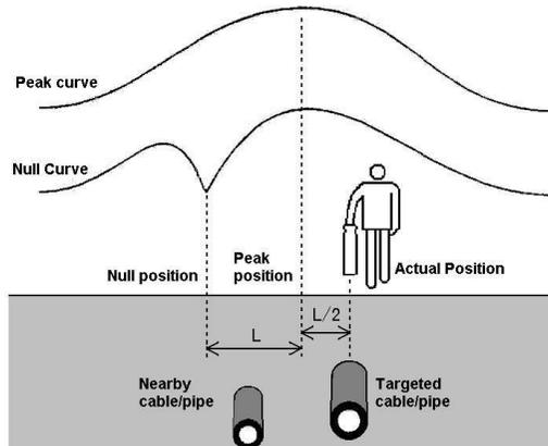
Fig.4.10 Positioning correction
