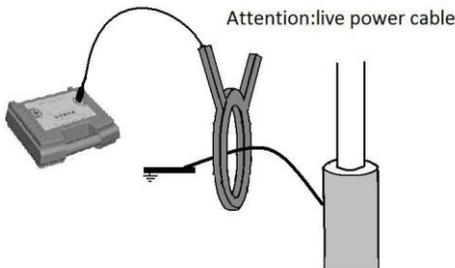
other sheath. Notice it when detection. For three cores belted cable, if not suitable to clamp the cable, clip the cable grounding line is also useful. But during some special situation, this will make signal feature unpredictable variation.
