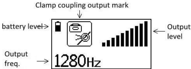
Fig.2.8 Clamp coupling output interface
