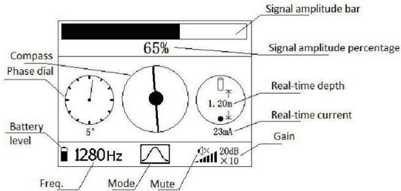
Fig.4.1 Pipe detection interface diagram
