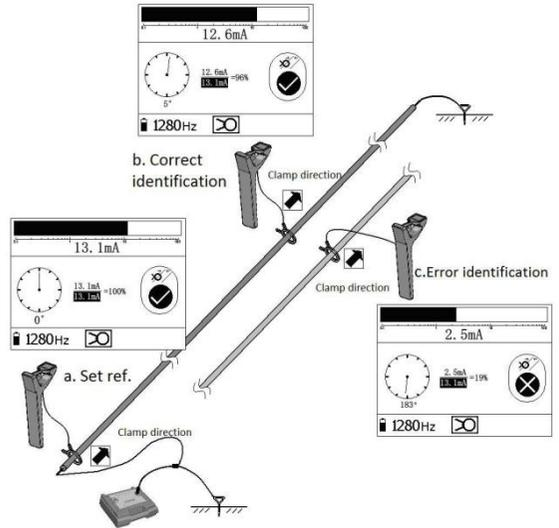
Fig.5.3 Clamp identification process
