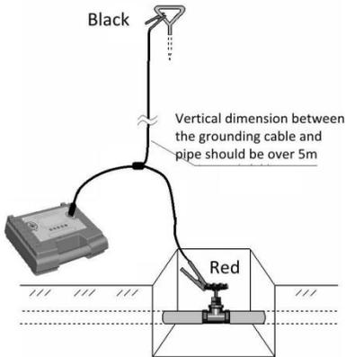
Connect the red alligator clip with the exposed metallic part of the pipe and connect the black alligator clip with the inserted grounding rod. If grounding cable is not long enough use the optional extending line.
