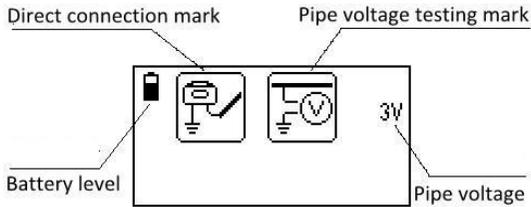
Fig.2.3 Pipe voltage measurement interface
