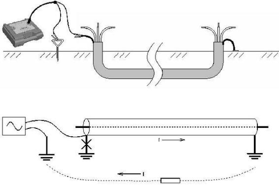
Fig.3.2 Sheath-Earth Method
