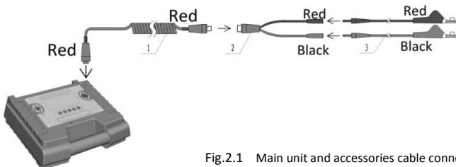
Fig.2.1 Main unit and accessories cable connection diagram
