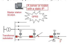
spontaneously or at regular intervals. At the same time, people can use a USB interface's wireless RF and interface software to read the real-time and fault-time data from GWFOL2-A16, or use master station SCADA and GPRS to achieve the on-site monitoring
