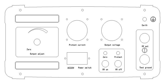
Fig.1 transmitter panel
