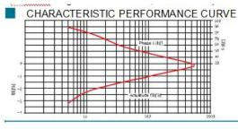
Ratio: 1000:1; Frequency: 50 Hz; Burden 1 Ohms;
