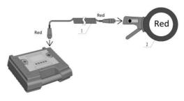
Fig.2.6 Clamp coupling accessories connection diagram
