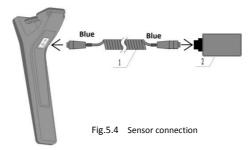
Please notice, sensor is used in the buried cable. Some bridge cables not suitable to direct contact can use the rod sensor.
