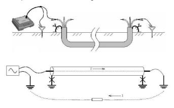
Fig.3.1 Conductor-Earth Connection Method
