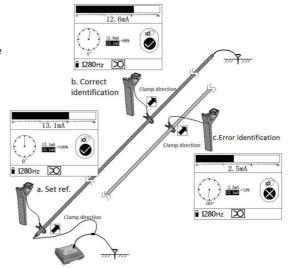
Fig.5.3 Clamp identification process
