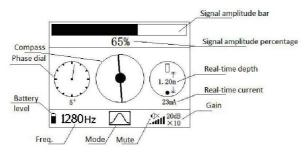
Fig.4.1 Pipe detection interface diagram
