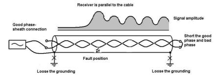
Fig.7.2 Phase to armor grounded fault pinpointing
