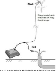
Fig.6.1 Connection for grounded fault pinpoint
