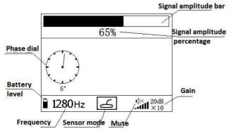
Fig.5.5 Sensor identification mode interface
