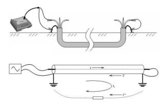
Fig.3.3 Phase-Sheath Method
