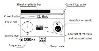
Fig.5.2 Clamp identification interface
