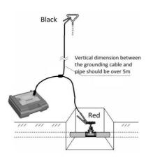
Connect the red alligator clip with the exposed metallic part of the pipe and connect the black alligator clip with the inserted grounding rod. If grounding cable is not long enough use the optional extending line.
