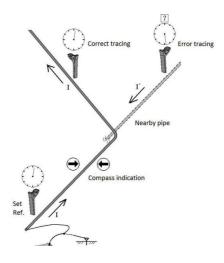
The process of Correct/Error indication as below Fig. 4.6
