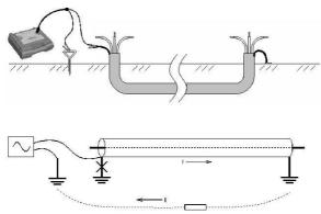
Fig.3.2 Sheath-Earth Method
