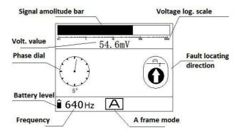
Fig.6.3 Interface for A frame fault location
