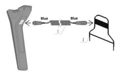
Fig.6.2 Connection for A frame
