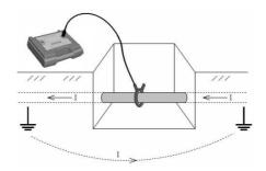
Fig.2.7 Clamp coupling mode wiring
