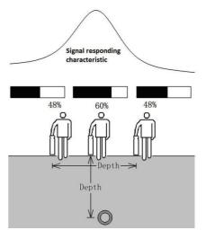
Fig.4.14 80% wide peak depth measurement
