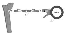
Fig.5.1 Receiving clamp connection
