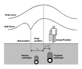
Fig.4.10 Positioning correction
