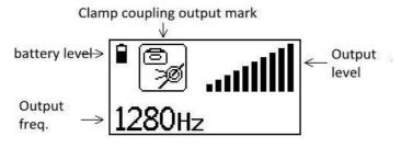
Fig. 2.8 Clamp coupling output interface
