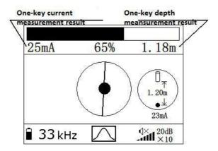
Fig.4.12 One-key depth and current measurement
