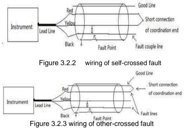
• In the wiring process of bridge test, there should not have any mistakes of the judgment of faults, the selection of good line and fault lines, the good short connection of core line in the coordination end, the wiring of the three clips. Otherwise, the testing is easily failed.
