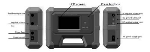
Fig.1 Transmitter appearance
