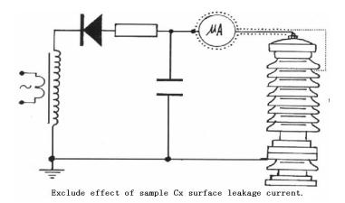
c. For sample such as zinc oxide, magnetic blow-out arrester, the grounding end can be breaked up; also can measure by connecting ammeter to the bottom (ground potential side) of test items. when we exclude effect of sample surface leakage current, we can use soft of bare copper wire in the sample to end the last laps around the shield ,and connect shielding line (see below)
