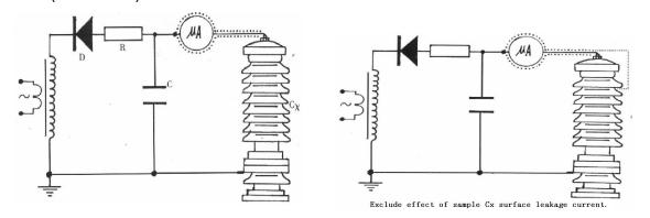
13. For small capacitive products , such as zinc oxide and lightning arrester , it discharges quickly through pressure resistance. For large capacitive products such as cable, while test voltage self discharging to the test voltage is below 20%, then it can discharge by supporting the discharging rod. Keep connect the grounding wire to the capacitive
