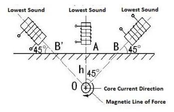
Illustration of 45 Degree Depth Measurement
