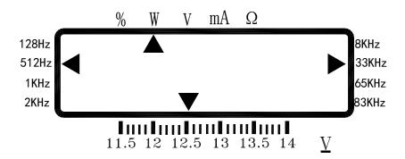
Working Frequency: When the frequency of the transmitter is selected, the corresponding triangular indicator light is on, and the available frequencies are 128Hz, 512Hz, 1KHz, 2KHz, 8KHz, 33KHz, 65KHz, 83KHz.
