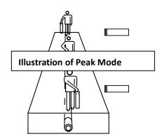
First of all, position the target pipeline. Generally, keep the receiver perpendicularly to ground with the receiver body pointing at the transmitter. If the signal is directly connected to the target pipeline, walk around the transmitter with the transmitter as the center and 5-10 meters Radius (if the inductive connectionis selected, the radius need be greater than 20 meters), adjust the sensitivity so that the receiver maintains a certain static signal.
