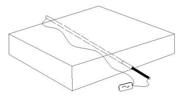
instead of starting from the complex underground pipelines. For example, if there are water pipes, gas pipes, power cables, etc. in a building, the signals should be applied from valves or other access points outside the building instead of signals from the building.
