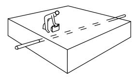
Place the transmitter on the "positive" side of the target line, and in the same pipeline
