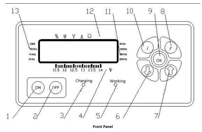
1&2.ON/OFF; 3.Charging Indicator; 4.Voltage Indicator; 5.Working Indicator; 6&7.Frequency Adjustment;
