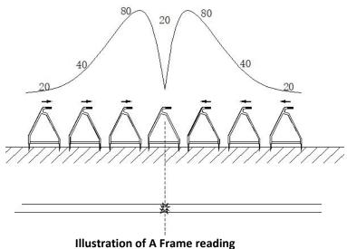
If the position of the pipeline cannot be determined during the fault point search, the mode key needs to be pressed at this time and the working mode need to be switched to the single horizontal coil, double horizontal coil or vertical coil to accurately position the target pipeline. After the positioning is completed, press the mode button again to select the external signal working mode and continue the fault point search.
