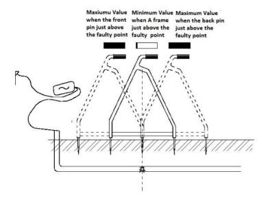
Illustration of Positioning Fault Point using A Frame
