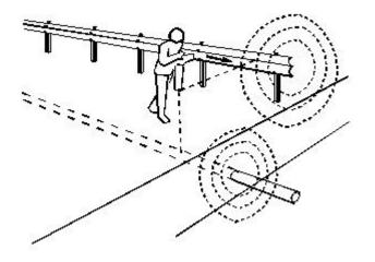
Illustration of Cable Detection of the Fence
