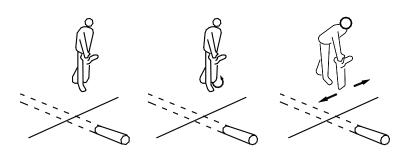
Use the peak mode to locate the pi Illustration of Locating the Pipe with Peak Mode
