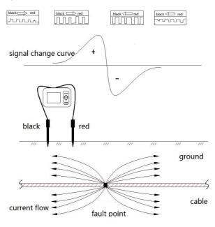
Fig.8 Step voltage pinpointing reference
