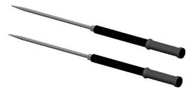
Fig.3 step-voltage probes
