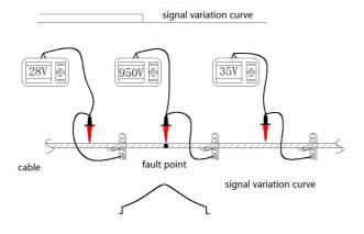
Fig.10 HV rod pinpointing section diagram
